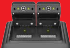
4 Channels & dual block 16-Well Design, can run two different programs independetly
